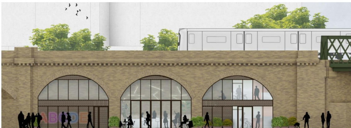
Figure 11: Proposed elevation of the three railway arches, showing the metal framed frontages to be installed, the central one of which would be brought into active reuse as part of a flexible retail/service/dining unit.
