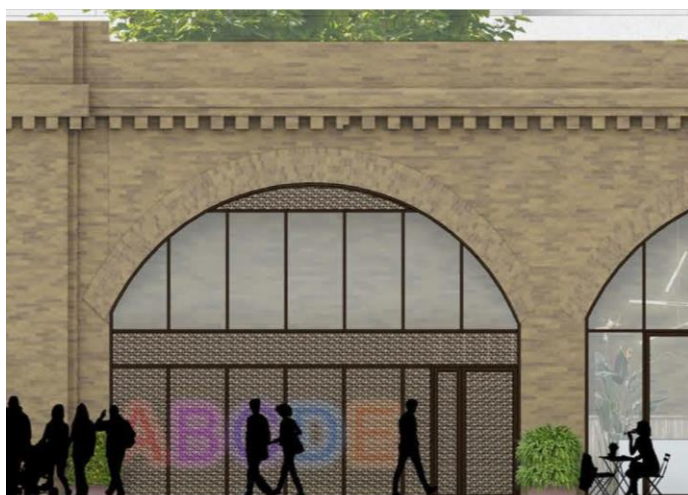
Image 50 (above): Elevation of the northern arch, showing indicatively how a scheme of lighting could be applied to the panelling.
